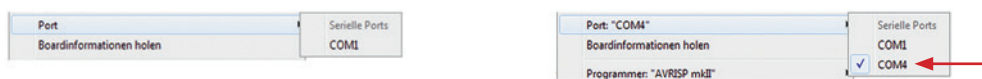
Fig. 22: Left: USB cable not connected, right: USB cable connected (virtual COM port selected)
