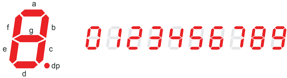
Fig. 31: The 7 segment indicator
